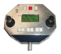
The seven movements are controlled by a control terminal shielded. It consists of a *stop* emergency button and a *mode selection*, two joysticks to control six movements (movements along the two axes of rotation and joystick itself) control buttons for opening and closing the clamp, two command buttons programming. A display screen allows the teleoperator to choose from various functions available and display different messages.
