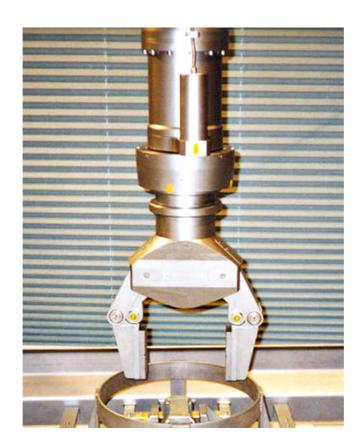
UNIVERSAL ARM is a mean of remote prehension moving along a vertical axis, usable in any cell equipped with a lifting device, for heavy interventions and handling of metal elements or not, irradiating or contaminated.
