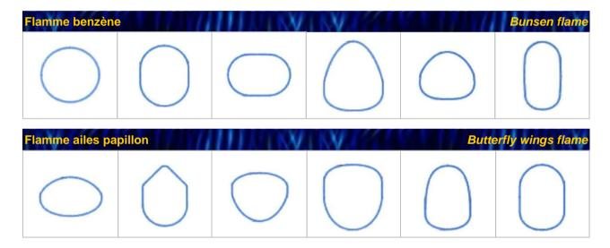
Orientation flame: the orientation of the flames is defined according to the use of the burner, here are few examples.
